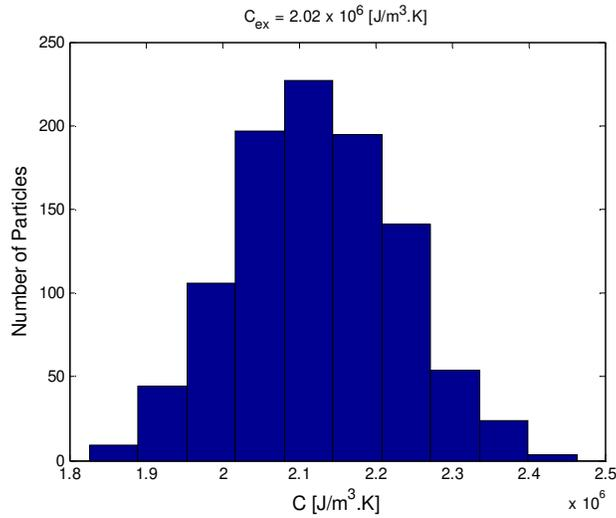
Figure 4: Histogram of the volumetric heat capacity estimated with Model 1 for case 1.
