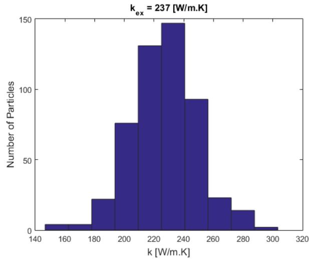
Figure 7: Histogram of the thermal conductivity estimated using Model 1 for case 2
