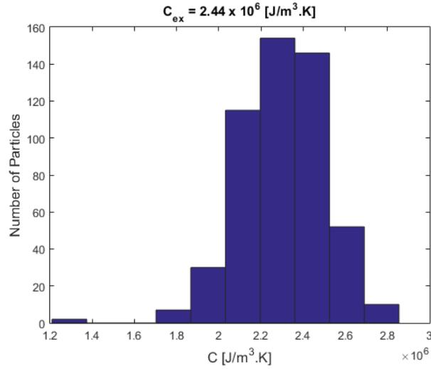
Figure 8: Histogram of the volumetric heat capacity estimated using Model 1 for case 2
