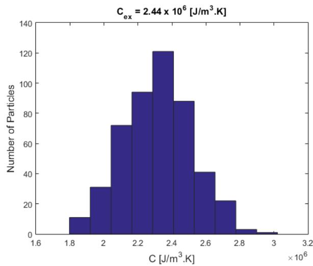
Figure 9: Histogram of the volumetric heat capacity estimated using Model 2 for case 2
