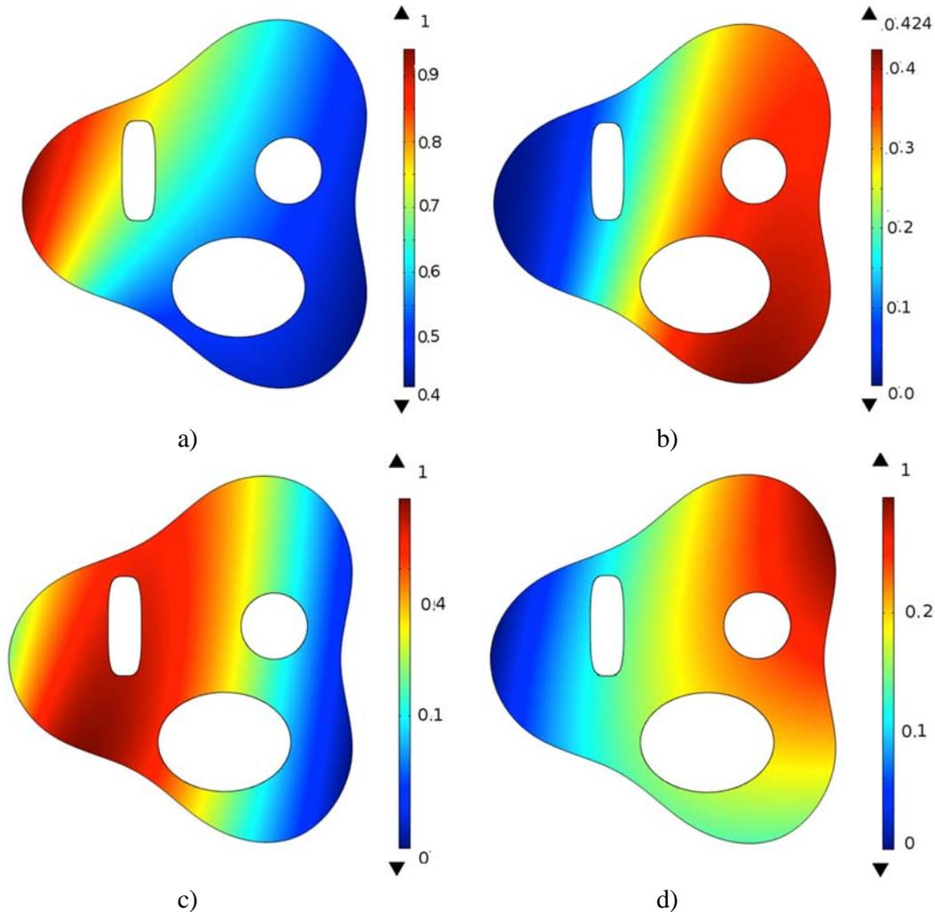
Figure 8. Case 3: Distribution of relative error in percents between exact thermal conductivity and converged conductivity with: a) 1% noise, b) 2% noise and c) 3% noise and d) relative error between exact heat capacity and converged heat capacity with 3% error
