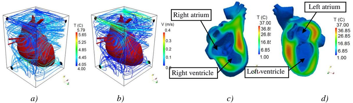
Figure 3. Results at 300 seconds: a) temperature distribution of external flow streamlines, b) speed distribution, c) temperature distribution inside the heart (1<sup>st</sup> cut-away view), and d) 2<sup>nd</sup> cut-away).
