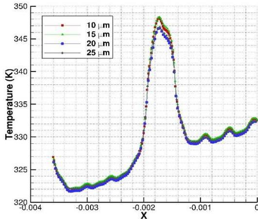
Figure 3. Temperature distribution along the sample line (Fig. 2a) for an entirely Silicon substrate.
