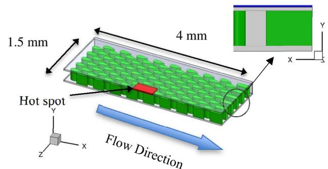
Figure 1. One half of a micro pin-fin cooling array and geometric dimensions as considered in this study
