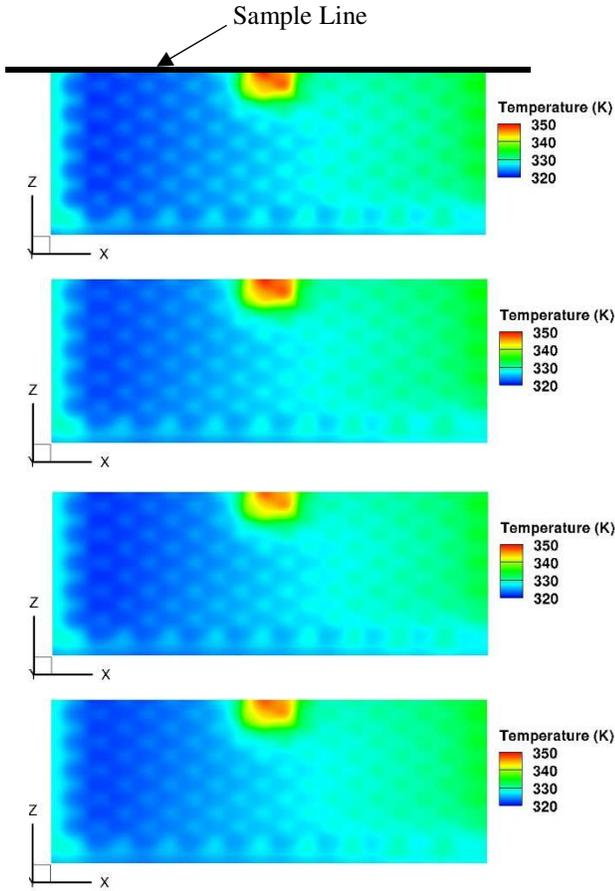
Figure 2. Temperature distribution on the top surface when using thermal conductivities for silicon for heat spreader thicknesses: a) 10  $\mu\text{m}$ , b) 15  $\mu\text{m}$ , c) 20  $\mu\text{m}$  and d) 25  $\mu\text{m}$ .
