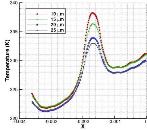
Figure 9. Case B: Temperature distribution along the sample line using isotropic GNP thin films.
