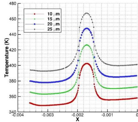
Figure 12. Case D: Temperature distribution along the sample line having thin films with in-plane GNPs.
