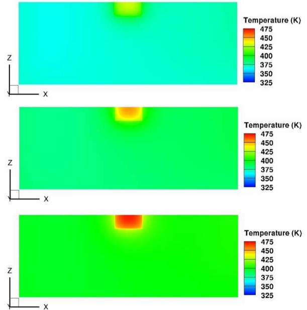
Figure 11. Case D: Temperature distribution on the top surface when using thermal conductivities for the GNP film thicknesses: a) 10  $\mu\text{m}$ , b) 15  $\mu\text{m}$ , c) 20  $\mu\text{m}$  and d) 25  $\mu\text{m}$ .
