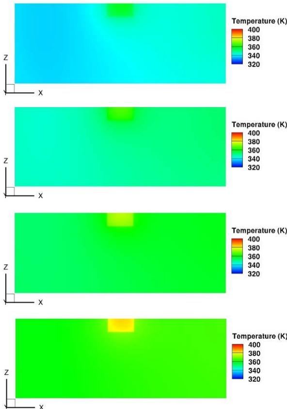
Figure 5. Case A: Temperature distribution on the top surface when using thermal conductivities for the GNP film thicknesses: a) 10  $\mu\text{m}$ , b) 15  $\mu\text{m}$ , c) 20  $\mu\text{m}$  and d) 25  $\mu\text{m}$ .
