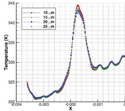
Figure 15. Case E: Temperature distribution along the sample line for preferential through-plane orientation of the GNPs in the films.
