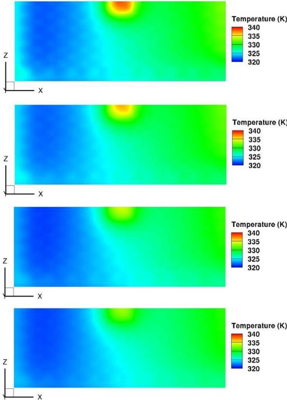
Figure 8. Case B: Temperature distribution on the top surface when using thermal conductivities for isotropic GNP film thicknesses: a) 10  $\mu\text{m}$ , b) 15  $\mu\text{m}$ , c) 20  $\mu\text{m}$  and d) 25  $\mu\text{m}$ .
