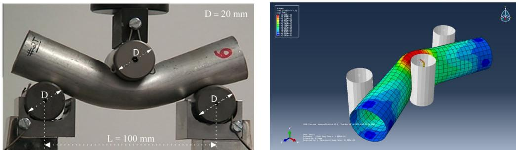
(a) Experimental set-up (Duarte *et al.*, 2015).
