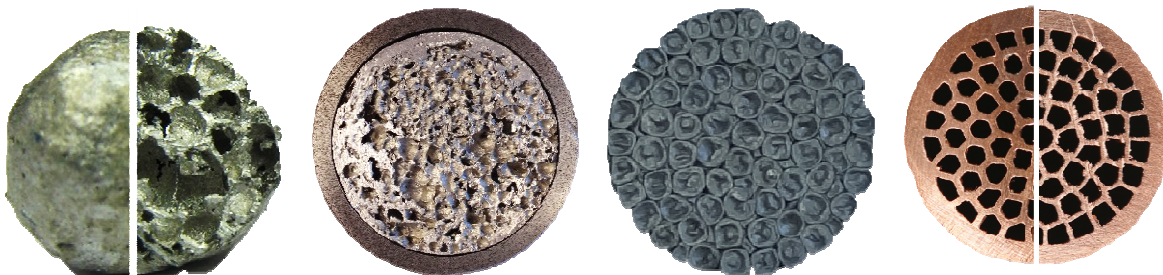
APM foam element, foam filled tube, MHSS and UniPore structure (from left to right).
