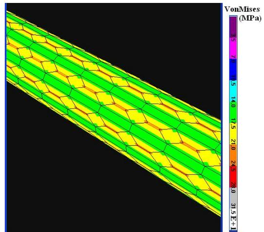
Fig. 6: Von Mises stresses of the rounded geometrical pattern
