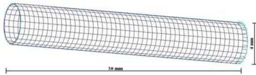
Fig. 2. Initial 3D finite element mesh.
