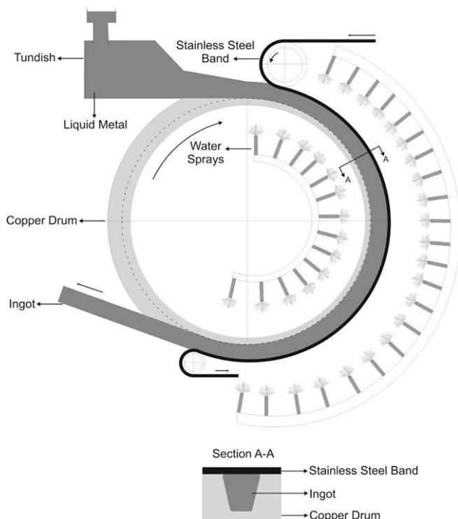
Fig. 1. Schematic of a rotary continuous caster.
