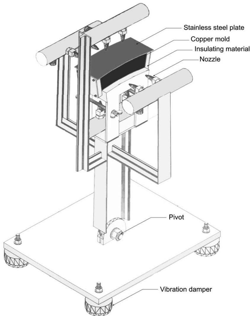
Fig. 2. Schematic representation of the experimental Properzi simulator.
