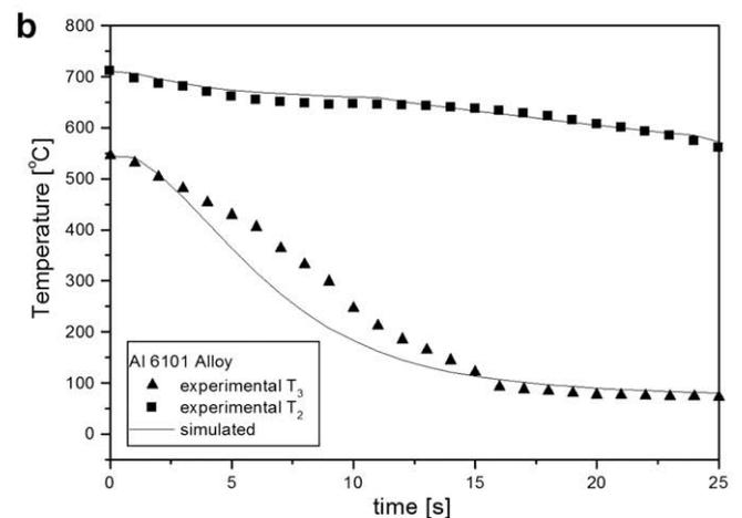
Fig. 8. Experimental and simulated temperatures. Al 6101 alloy (a) positions  $T_1$  (ingot top),  $T_4$  (ingot bottom) and  $T_5$  (mold bottom) (b) positions  $T_2$  (ingot lateral) and  $T_3$  (mold lateral).
