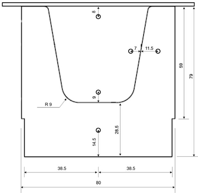
Fig. 4. Mold dimensions (mm) and thermocouples positions.
