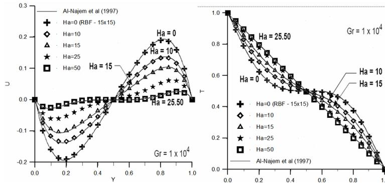
Figure 1. Velocity and temperature profiles for 15x15 RBF centers.
