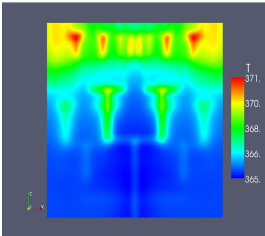
**Figure 14.** Top surface temperature field for the Pareto optimized 5-floor cooling network configuration no. 92 (lowest amount of heat removed).
