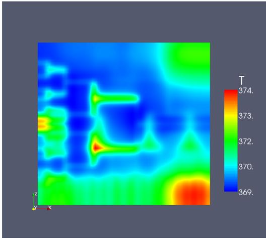
**Figure 10.** Top surface temperature field for the Pareto optimized 4-floor cooling network configuration no. 23 (lowest amount of heat removed).
