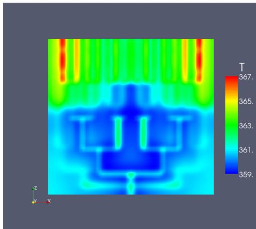
**Figure 5.** Top surface temperature field for the Pareto optimized 3-floor cooling network configuration no. 38 (high amount of heat removed).
