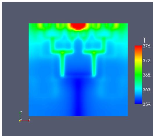
**Figure 7.** Top surface temperature field for the Pareto optimized 3-floor cooling network configuration no. 49 (low amount of heat removed).
