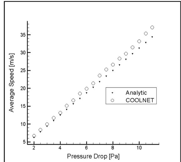
**Figure 2.** Validation of COOLNET for Poiseuille incompressible laminar flow test case.
