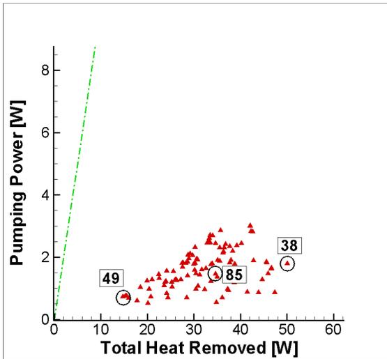
**Figure 4.** Pumping power vs. total heat removed for all Pareto-optimal solutions using a 3-floor cooling configuration.
