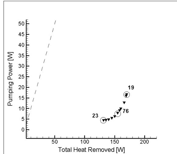
**Figure 9.** Pareto optimized solutions for a 4-floor configuration, 400 W/cm<sup>2</sup> uniform heating load, with each floor having different feeding orientation.
