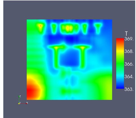
**Figure 15.** Top surface temperature field for the Pareto optimized 5-floor cooling network configuration no. 70 (highest amount of heat removed).
