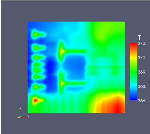
**Figure 12.** Top surface temperature field for the Pareto optimized 4-floor cooling network configuration no. 19 (highest amount of heat removed).
