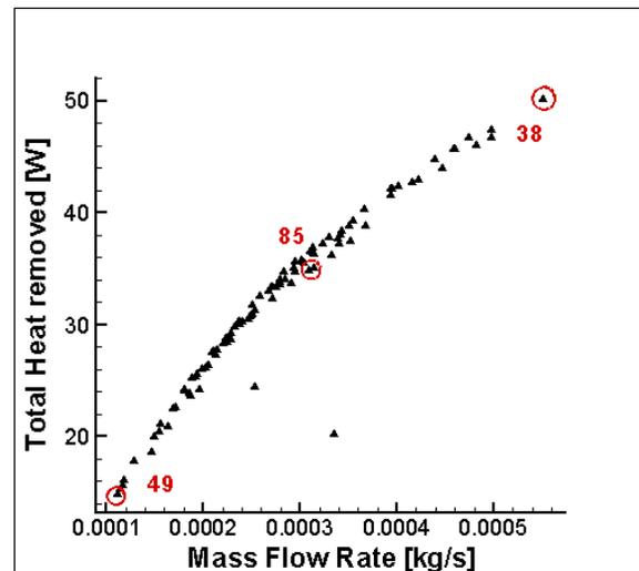
**Figure 3.** Heat removed vs. mass flow rate for Pareto-optimized solutions using a 3-floor cooling configuration.
