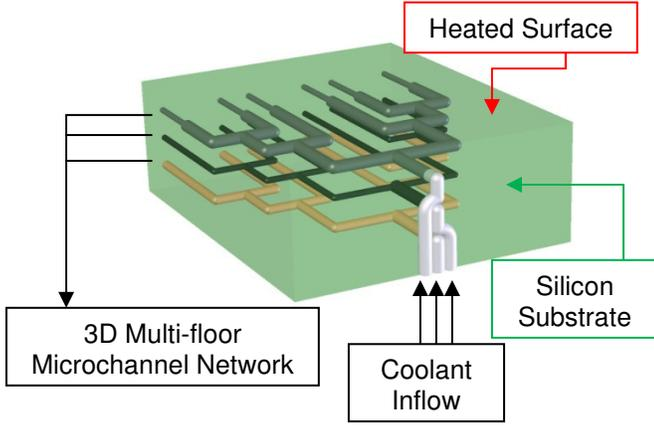
Figure 1. Sample 3D microchannel network.
