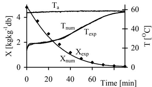
Fig. 8. The mid-plane temperature,  $T$ , the temperature of the drying air,  $T_a$ , and the volume-averaged moisture content,  $X$ , changes during the drying of a potato slice
