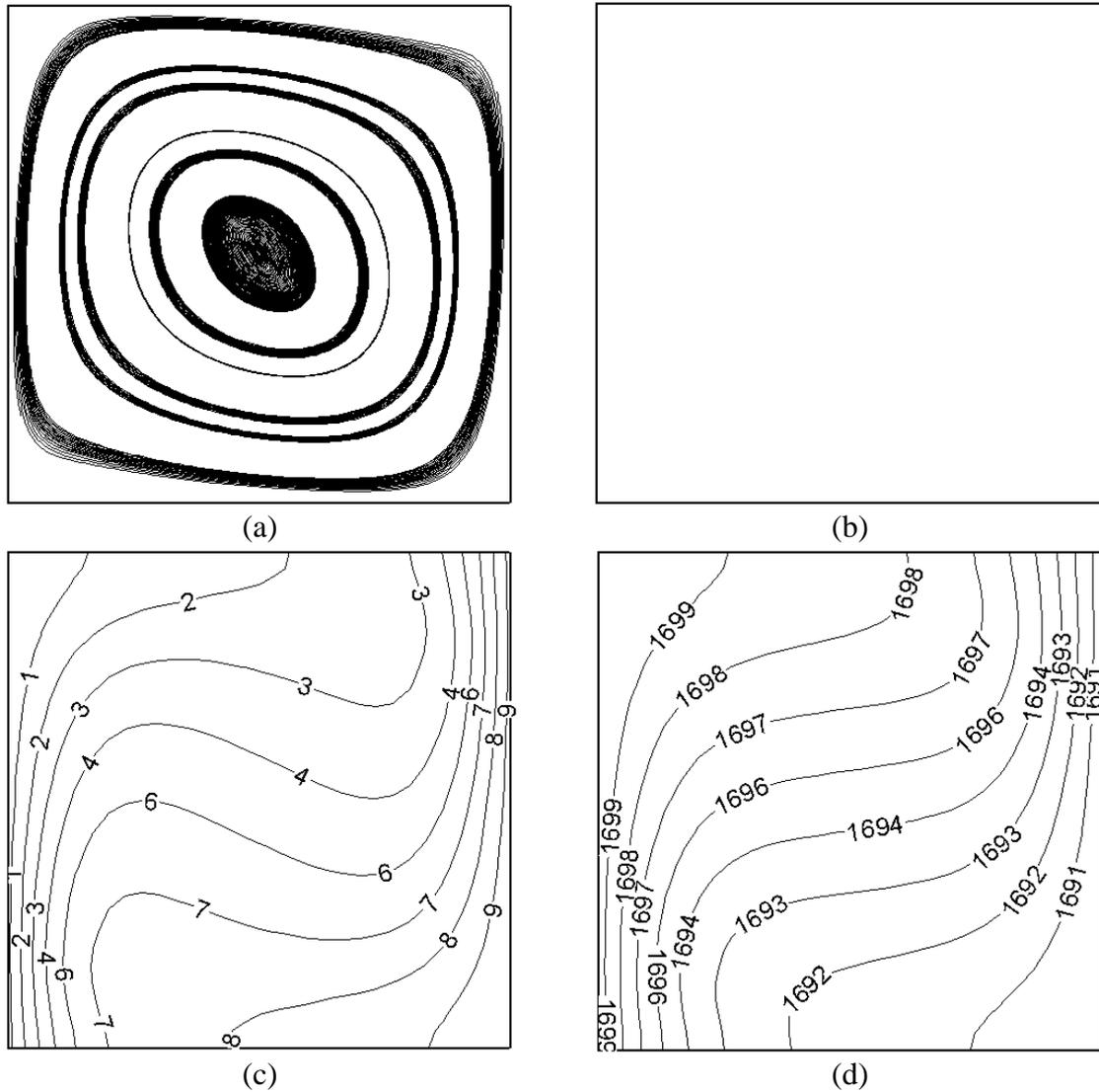
Figure 9: Streamlines (a), magnetic flux lines (b), iso-concentration lines (c) and isotherms (d) with no applied magnetic field ( $\mathbf{B} = 0$ )
