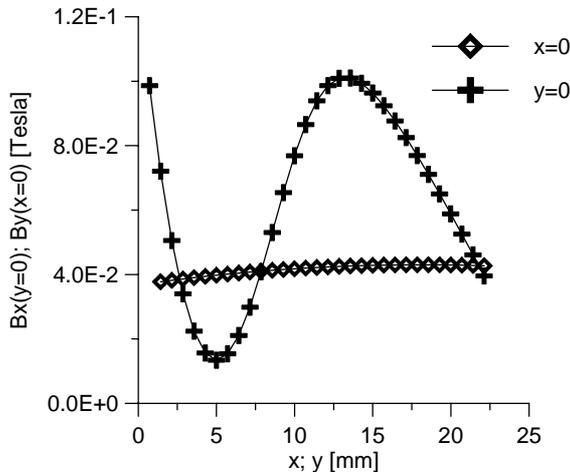
Figure 11: Optimized magnetic boundary conditions at  $x = 0$  and  $y = 0$  with the estimation of magnetic flux  $\mathbf{B}$  at six points per boundary
