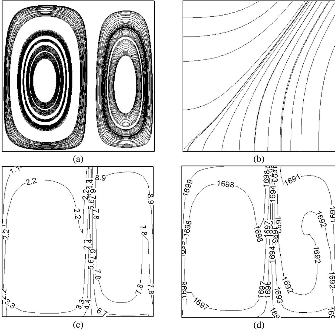
Figure 10: Streamlines (a), magnetic flux lines (b), iso-concentration lines (c) and isotherms (d) resulting from magnetic flux  $\mathbf{B}$  optimized at six points per boundary.
