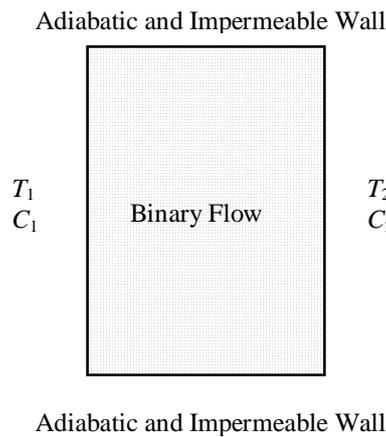
Figure 1: Geometry and boundary conditions for the thermosolutal analysis problem
