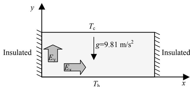
Figure 4.5.1 - Geometry and boundary conditions for EHD
