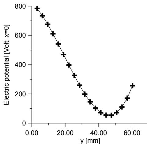
Figure 4.5.6. Solidification case: optimized electric potential boundary conditions at  $x = 0$  with  $Ra = 1.9 \times 10^4$  and estimation of  $E$  at six points
