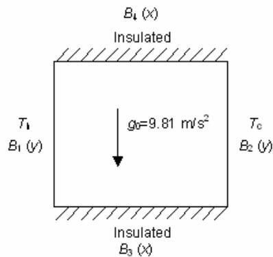
Figure 4.4.1 - Geometry and boundary conditions for MHD
