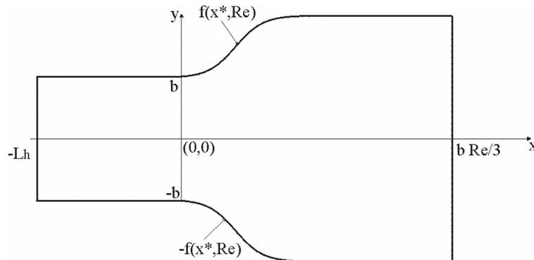
Figure 4.2.1 – Geometry for the channel with smooth expansion
