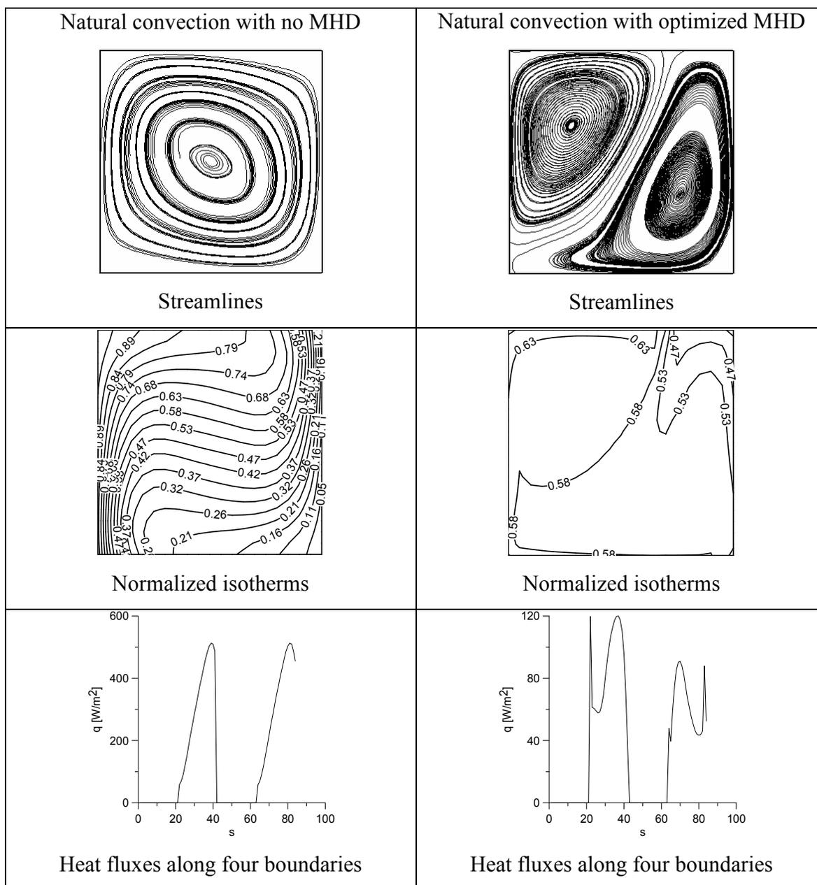
Figure 4.4.2 - Natural convection; results of analysis with no magnetic field (left column) and results with optimized magnetic boundary conditions (right column) for  $Ra = 10^5$ . The parameter  $s$  is measured counterclockwise along the boundaries of the rectangular container starting from lower the left corner.
