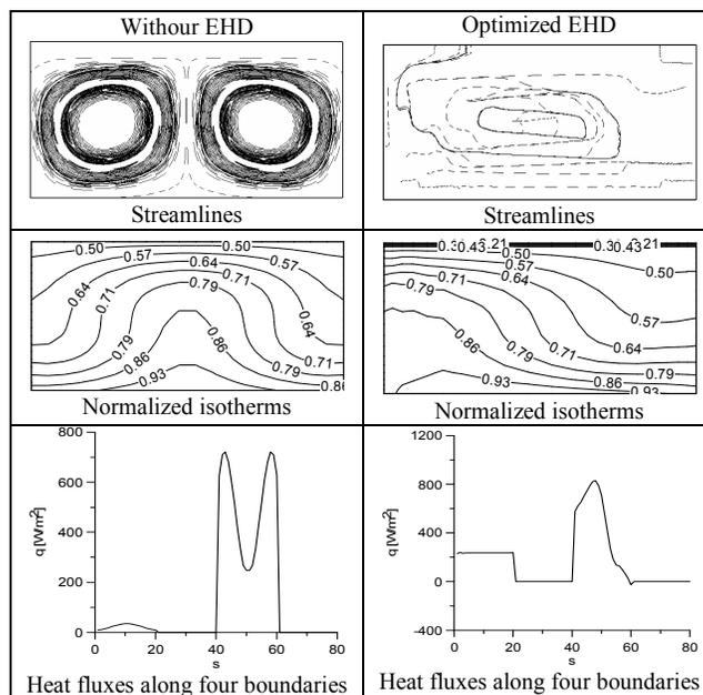
Figure 4.5.5. Natural convection with solidification; results of analysis with no electric field (left column) and results of optimized electric boundary conditions (right column) for  $Ra = 1.9 \times 10^4$ . The parameter  $s$  is measured counterclockwise along the boundaries of the rectangular container starting from lower left corner
