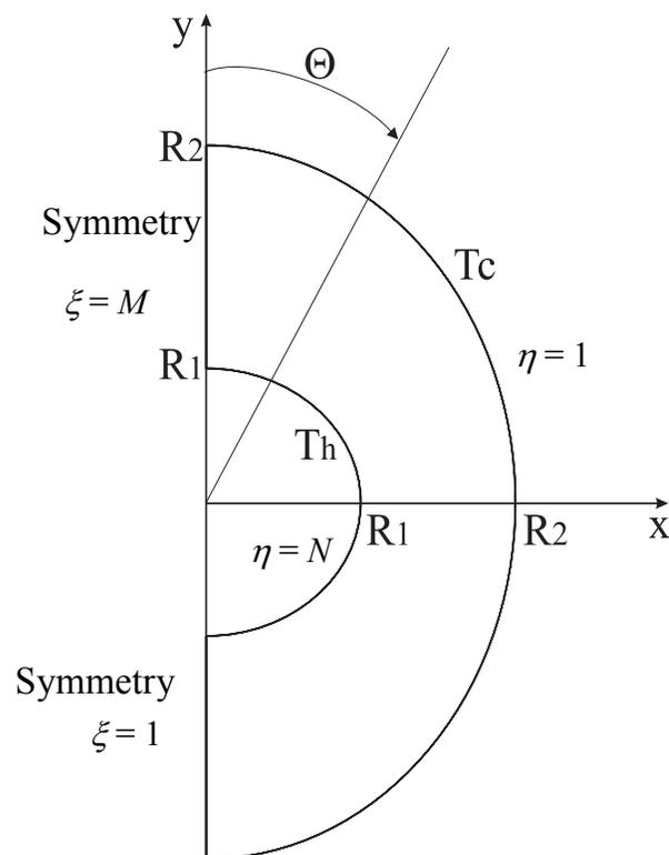
Figure 4.3.1 – Geometry for the irregular cavity
