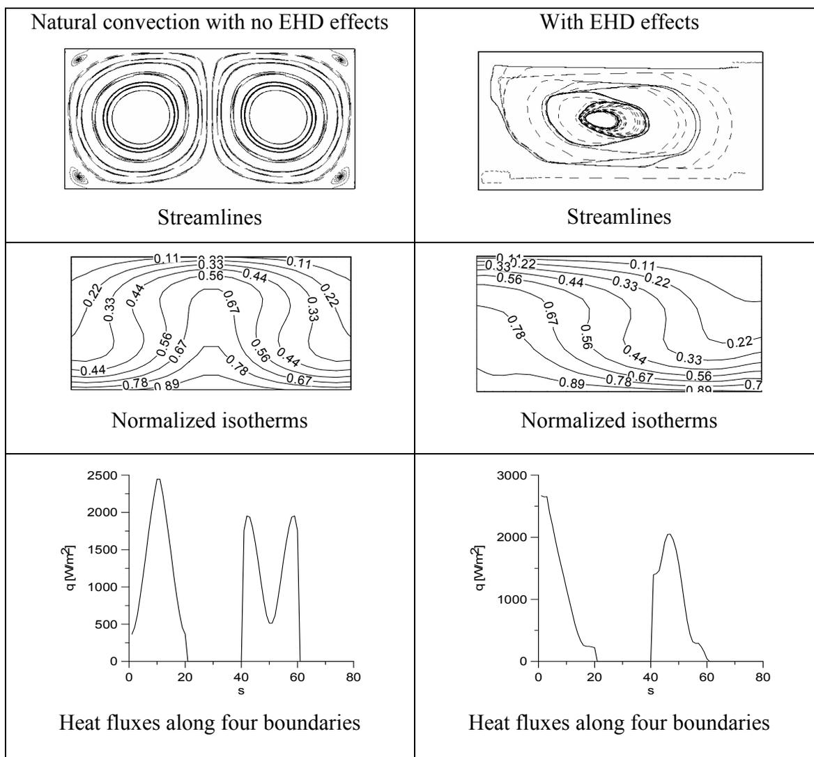
Figure 39 - Natural convection with no solidification; results of analysis with no electric field (left column) and results of optimized electric boundary conditions (right column) for  $Ra = 1.9 \times 10^4$ . The parameter  $s$  is measured counterclockwise along the boundaries of the rectangular container starting from lower left corner
