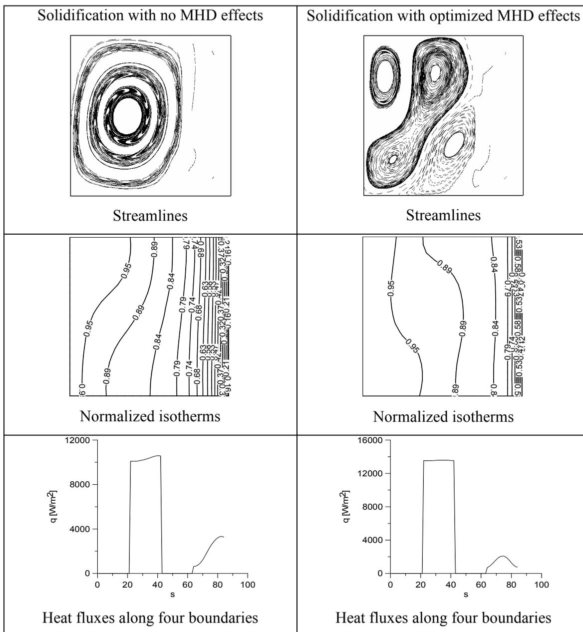
Figure 4.4.5 - Natural convection with solidification; results of analysis with no magnetic field (left column) and results with optimized magnetic boundary conditions (right column) for  $Ra = 10^5$ . The parameter  $s$  is measured counterclockwise along the boundaries of the rectangular container starting from the lower left corner
