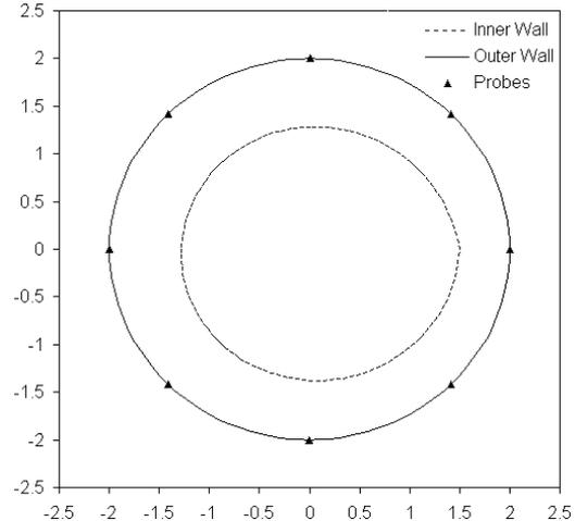
Fig. 2: Asymmetric test geometry: target shape of the inner surface and the outer surface (circle of radius 2.0 m) of the furnace wall with indication of the locations of eight temperature and heat flux probes.
