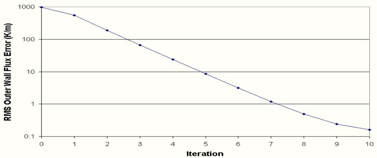
Fig. 9. Asymmetric case: convergence history of the RMS error of the outer surface heat flux.
