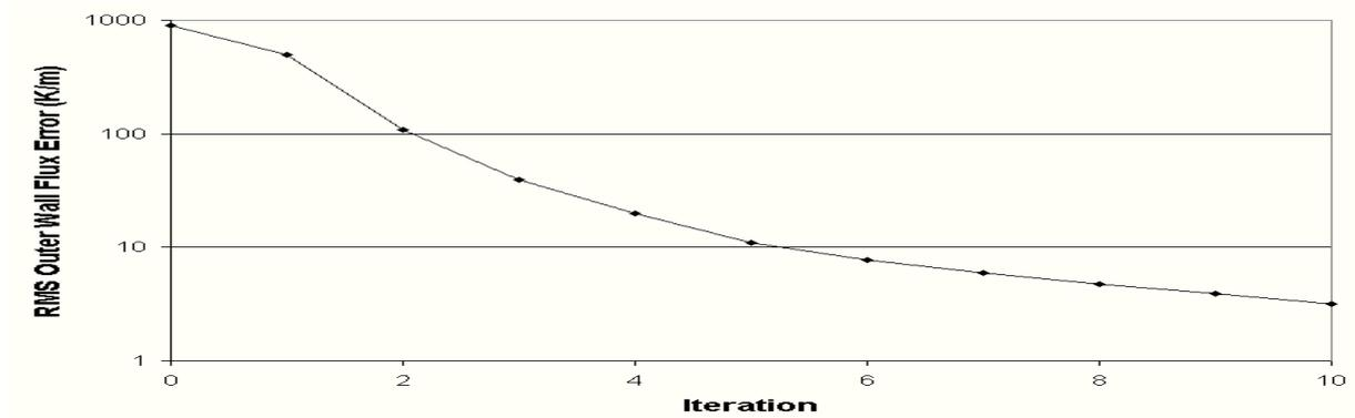
Fig. 5. Symmetric case: convergence history of the RMS error of the outer surface heat flux.
