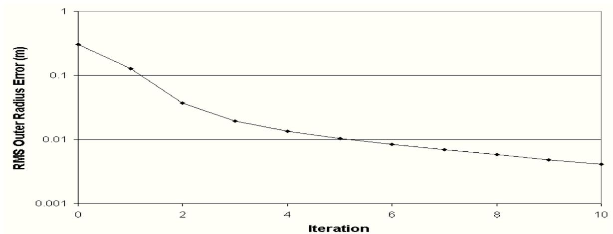
Fig. 6. Symmetric case: convergence history of the RMS error of inner surface geometry.
