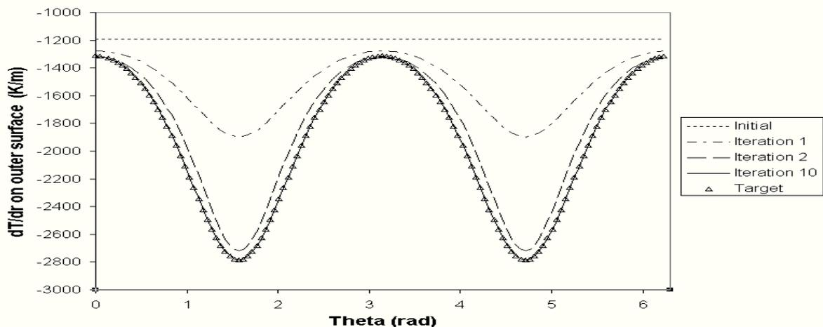
Fig. 3. Symmetric case: convergence history of the outer surface heat flux.
