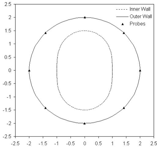
Fig. 1: Symmetric test geometry: target shape of the inner surface (vertical oval) and the outer surface (circle of radius 2.0 m) of the furnace wall with indication of the locations of eight temperature and heat flux probes.
