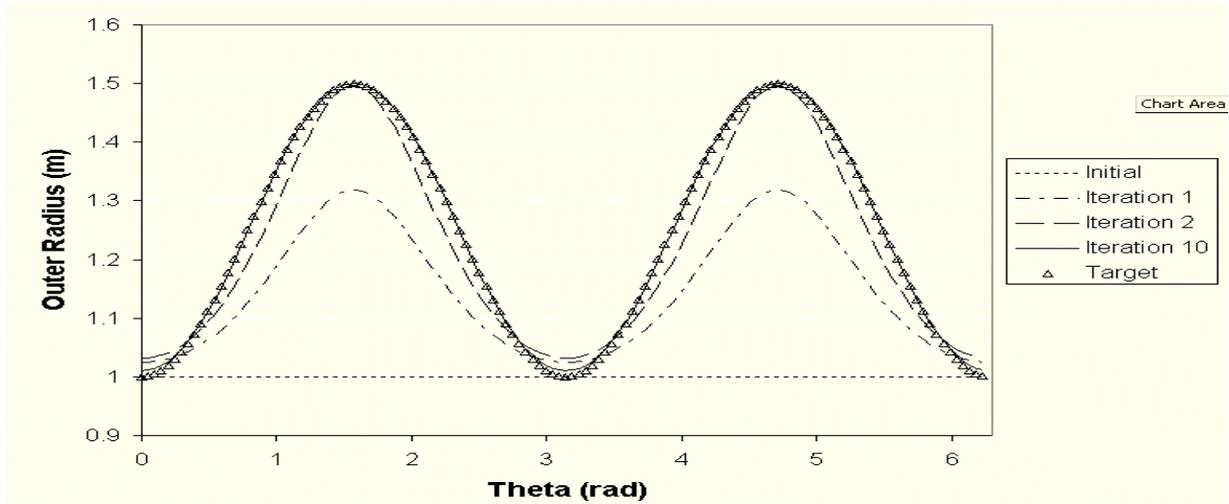
Fig. 4. Symmetric case: convergence history of the inner surface geometry.
