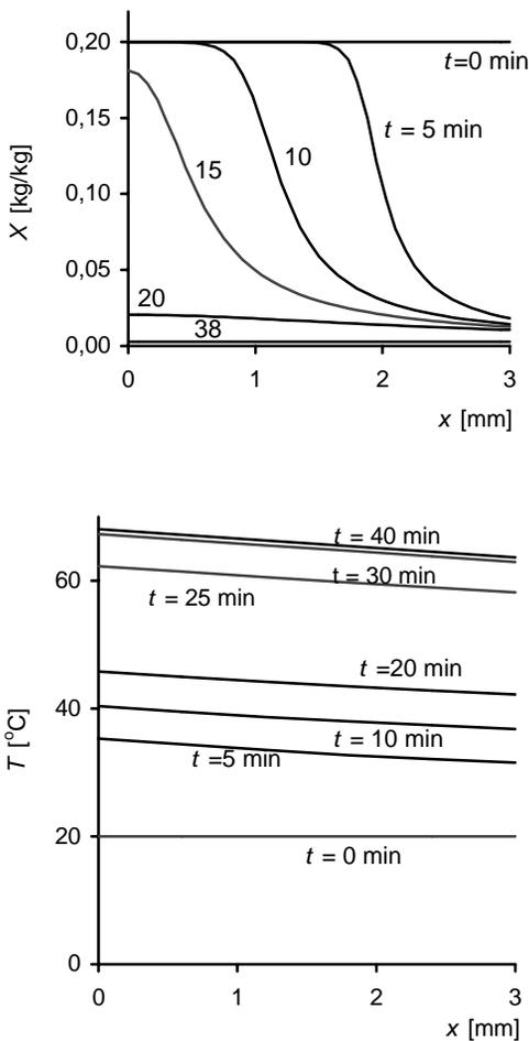
Fig.7. Transient moisture content and temperature profiles in the case of the contact drying experiment
