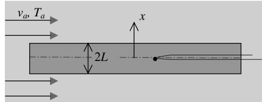
Fig. 1. Scheme of the convective drying experiment
