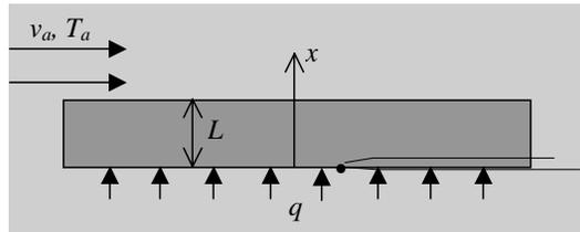
Fig. 2. Scheme of the contact drying experiment
