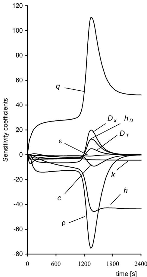
Fig.5. Relative sensitivity coefficients for the contact drying experiment
