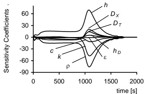
Fig.3. Relative sensitivity coefficients for the convective drying experiment
