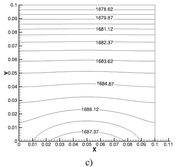
Figure 2. Results for test case no. 1 (full gravity and no magnetic field); a) streamlines, b) velocity magnitudes, c) isotherms.
