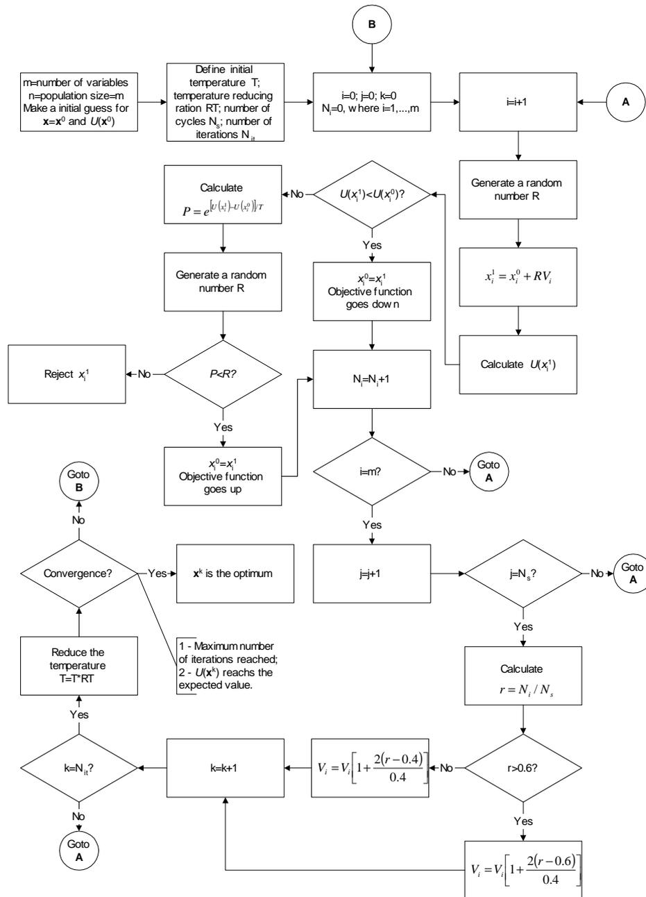
Figure 8. Iterative procedure for the Simulated Annealing Method.
