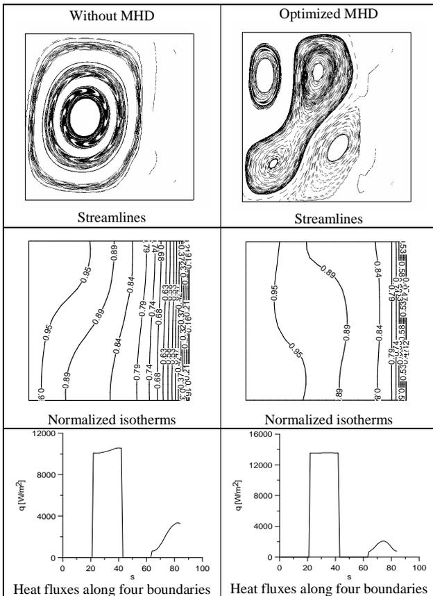
Figure 25. Natural convection with solidification; results of analysis with no magnetic field (left column) and results with optimized magnetic boundary conditions (right column) for  $Ra = 10^5$ . The parameter  $s$  is measured counterclockwise along the boundaries of the rectangular container starting from the lower left corner.
