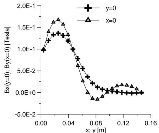
Figure 23. Natural convection; optimized magnetic boundary conditions at  $x = 0$  and  $y = 0$  with the estimation of  $\mathbf{B}$  at six points per boundary.
