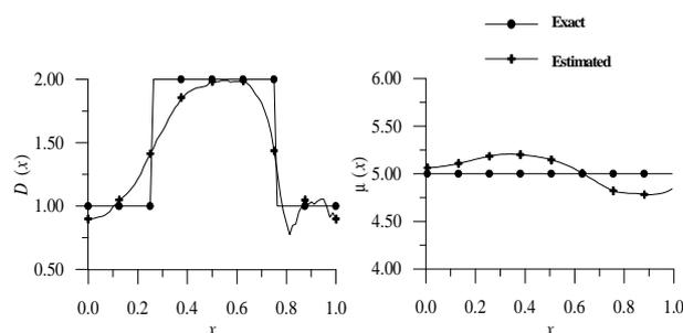
Figure 10. Estimation of  $\mu(x)$  and  $D(x)$  obtained by the CGM with two non-intrusive sensors with standard deviation ( $\sigma = 0.01 Y_{max}$ ).
