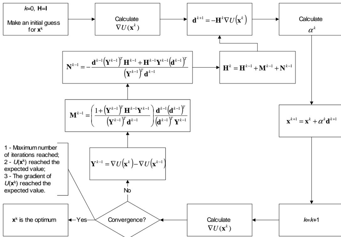
Figure 4. Iterative procedure for the BFGS Method.
