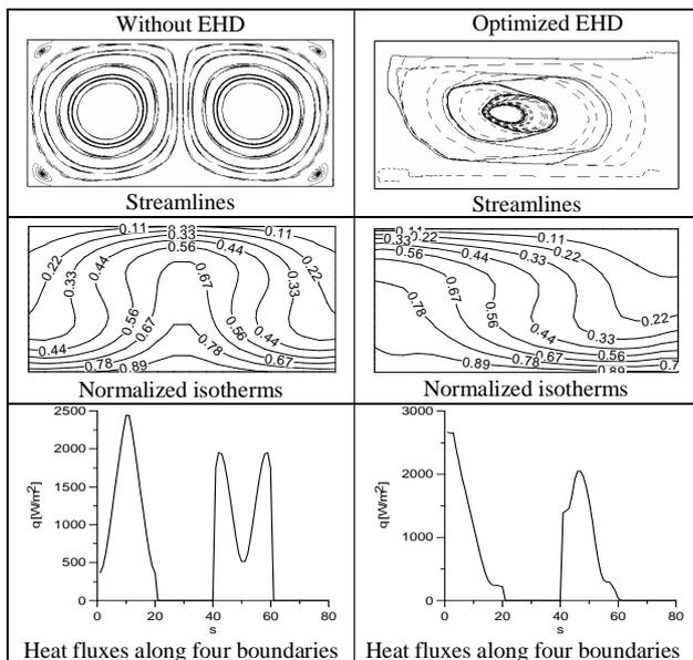
Figure 29. Natural convection with no solidification; results of analysis with no electric field (left column) and results of optimized electric boundary conditions (right column) for  $Ra = 1.9 \times 10^4$ . The parameter  $s$  is measured counterclockwise along the boundaries of the rectangular container starting from lower left corner.
