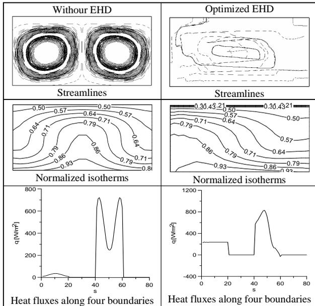
Figure 32. Natural convection with solidification; results of analysis with no electric field (left column) and results of optimized electric boundary conditions (right column) for  $Ra = 1.9 \times 10^4$ . The parameter  $s$  is measured counterclockwise along the boundaries of the rectangular container starting from lower left corner.
