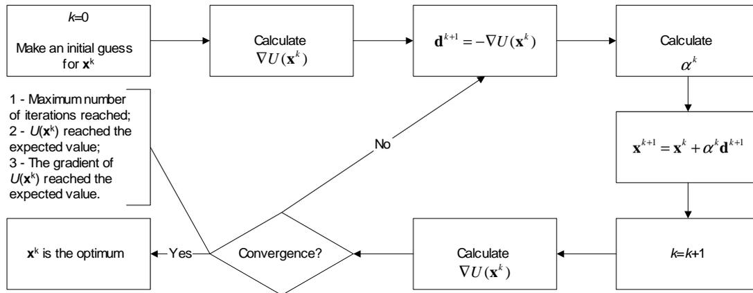
Figure 1. Iterative procedure for the Steepest Descent Method.
