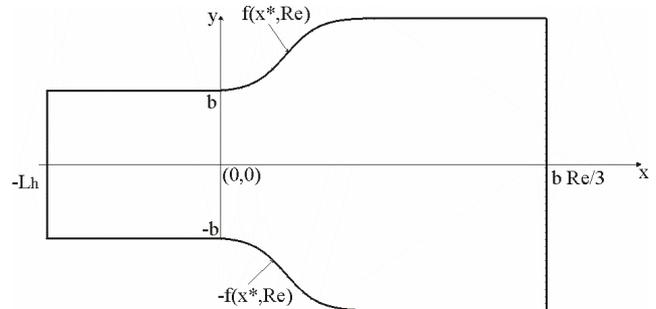
Figure 17. Geometry for the channel with smooth expansion.
