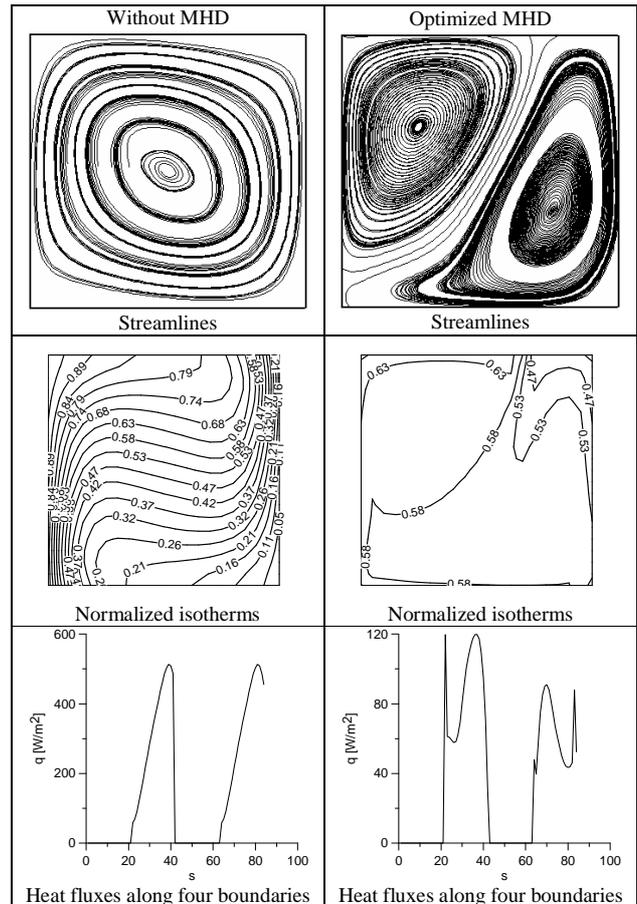
Figure 22. Natural convection; results of analysis with no magnetic field (left column) and results with optimized magnetic boundary conditions (right column) for  $Ra = 10^5$ . The parameter  $s$  is measured counterclockwise along the boundaries of the rectangular container starting from lower the left corner.
