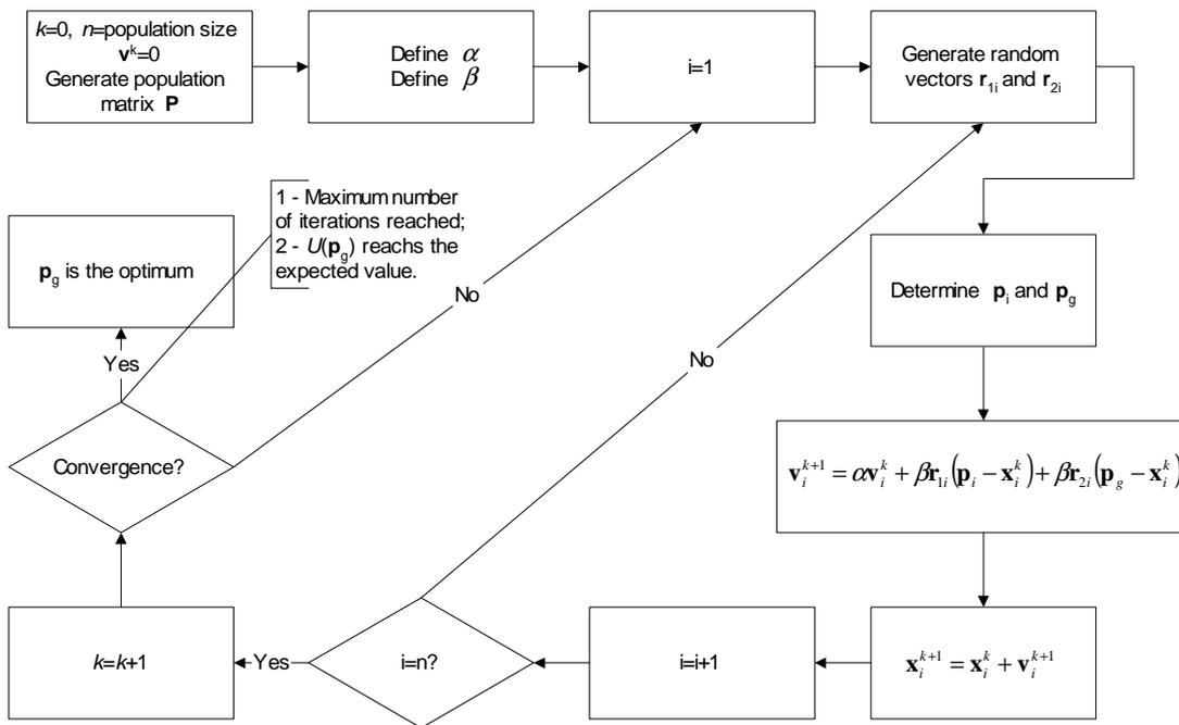
Figure 6. Iterative procedure for the Particle Swarm Method.
