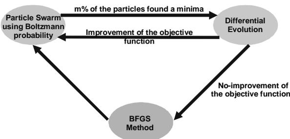
Figure 9. Global procedure for the Hybrid Method.
