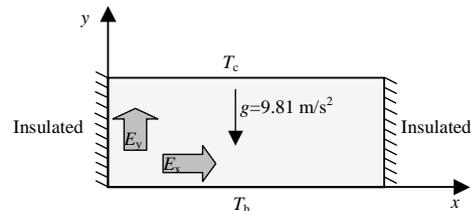
Figure 28. Geometry and boundary conditions for EHD.
