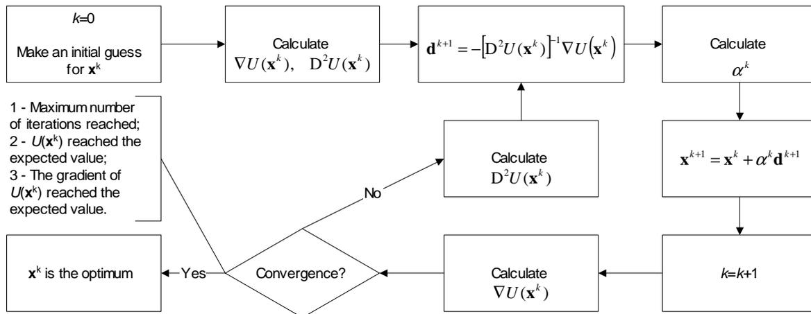
Figure 3. Iterative procedure for the Newton-Raphson Method.
