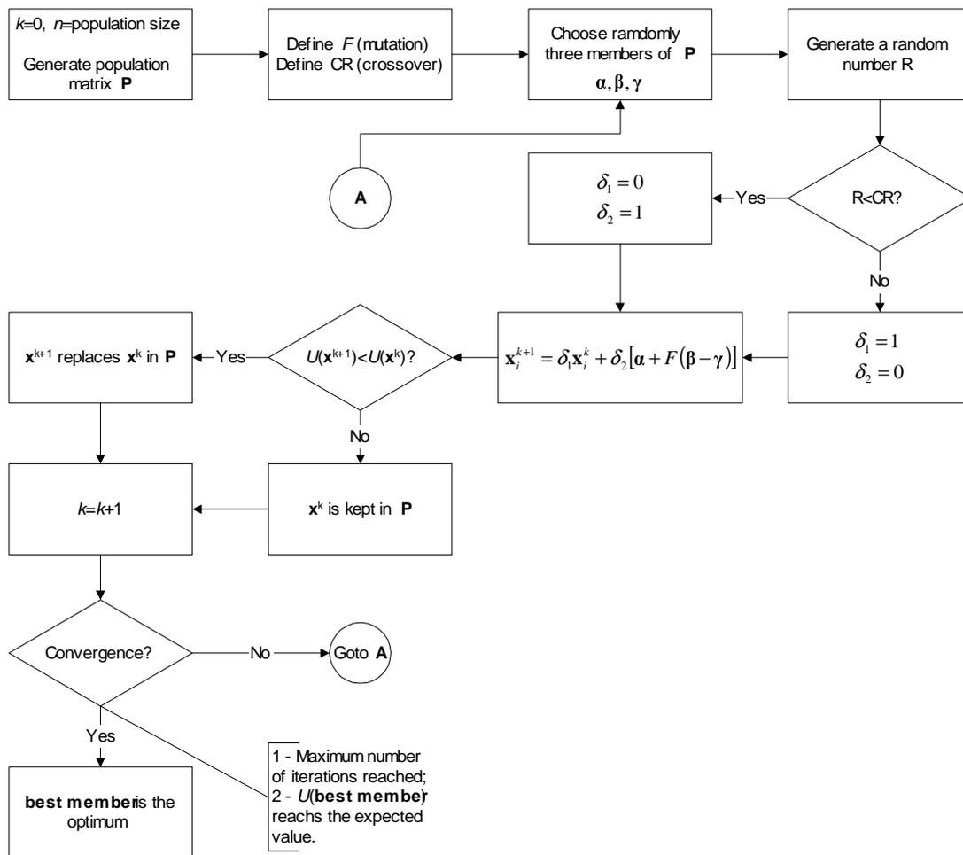
Figure 5. Iterative procedure for the Differential Evolution Method.
