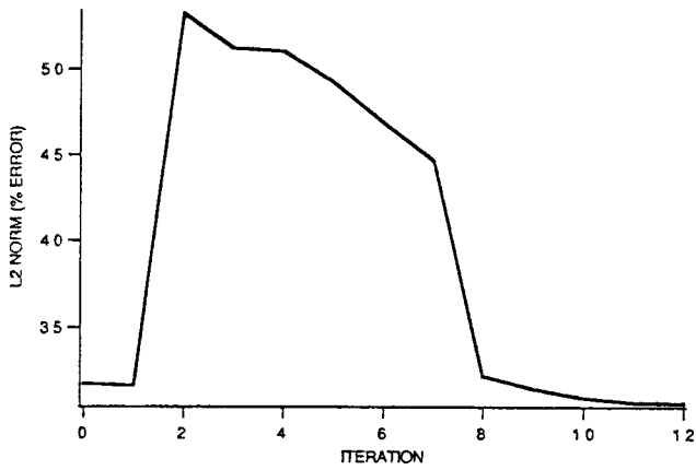
Figure 9. Coated turbine blade with T=600 K on each hole: convergence history (percentage of the integrated heat flux error on the outer boundary versus number of optimization cycles).
