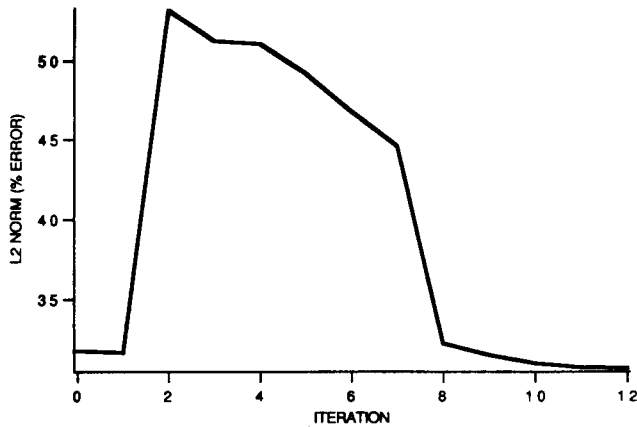
Fig. 9 Coated turbine blade airfoil with T = 600 K specified on each hole—convergence history (percentage of the integrated heat flux error on the outer boundary vs number of optimization cycles). Outer surface thermal conditions as in Figs. 5 and 6.
