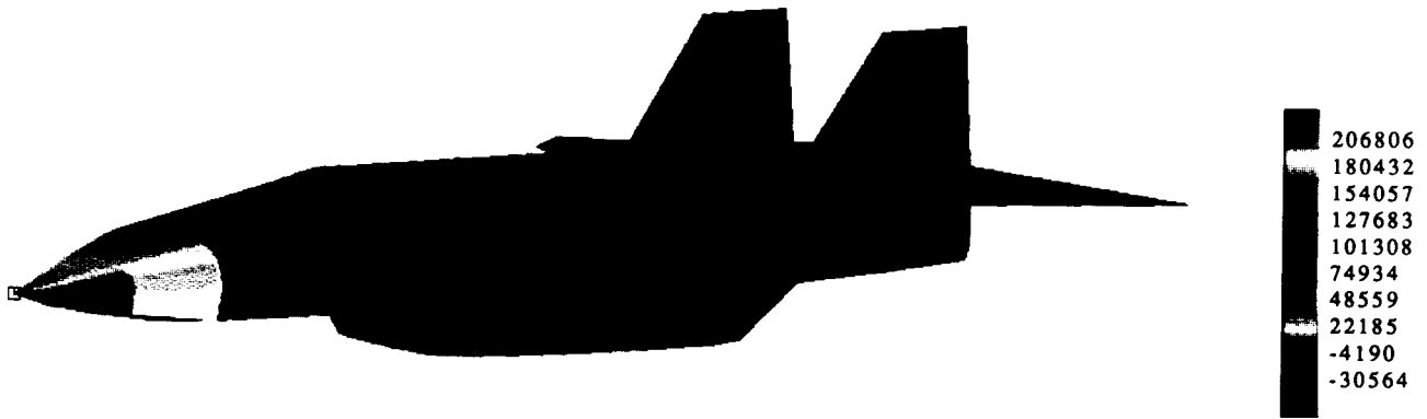
Figure 5. Original configuration (with pressure distribution) for the hypersonic plane.
