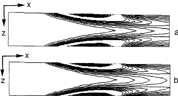
Fig. 11 Isotherms in straight duct with solidification ( y^* = 0.5, g = 0.01g_0 ): a) Ht = 10 ; b) Ht = 30 .
