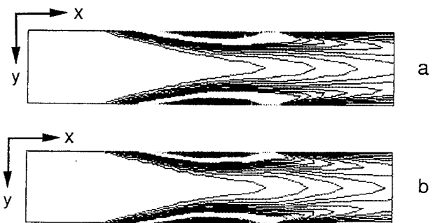
Fig. 12 Isotherms in straight duct with solidification ( z^* = 0.5, g = 0.01g_0 ): a) Ht = 10 ; b) Ht = 30 .
