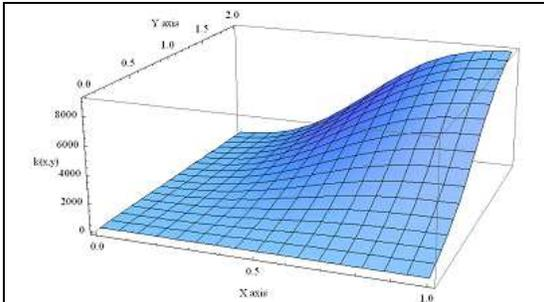
Figure 8. Thermal conductivity distribution using optimized four coefficients.
