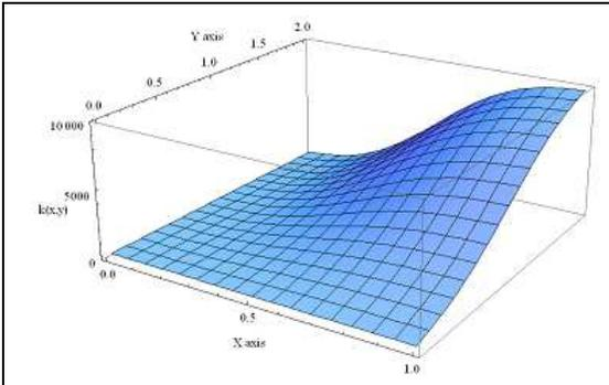
Figure 6. Actual distribution of thermal conductivity for case 2 (equation 13).
