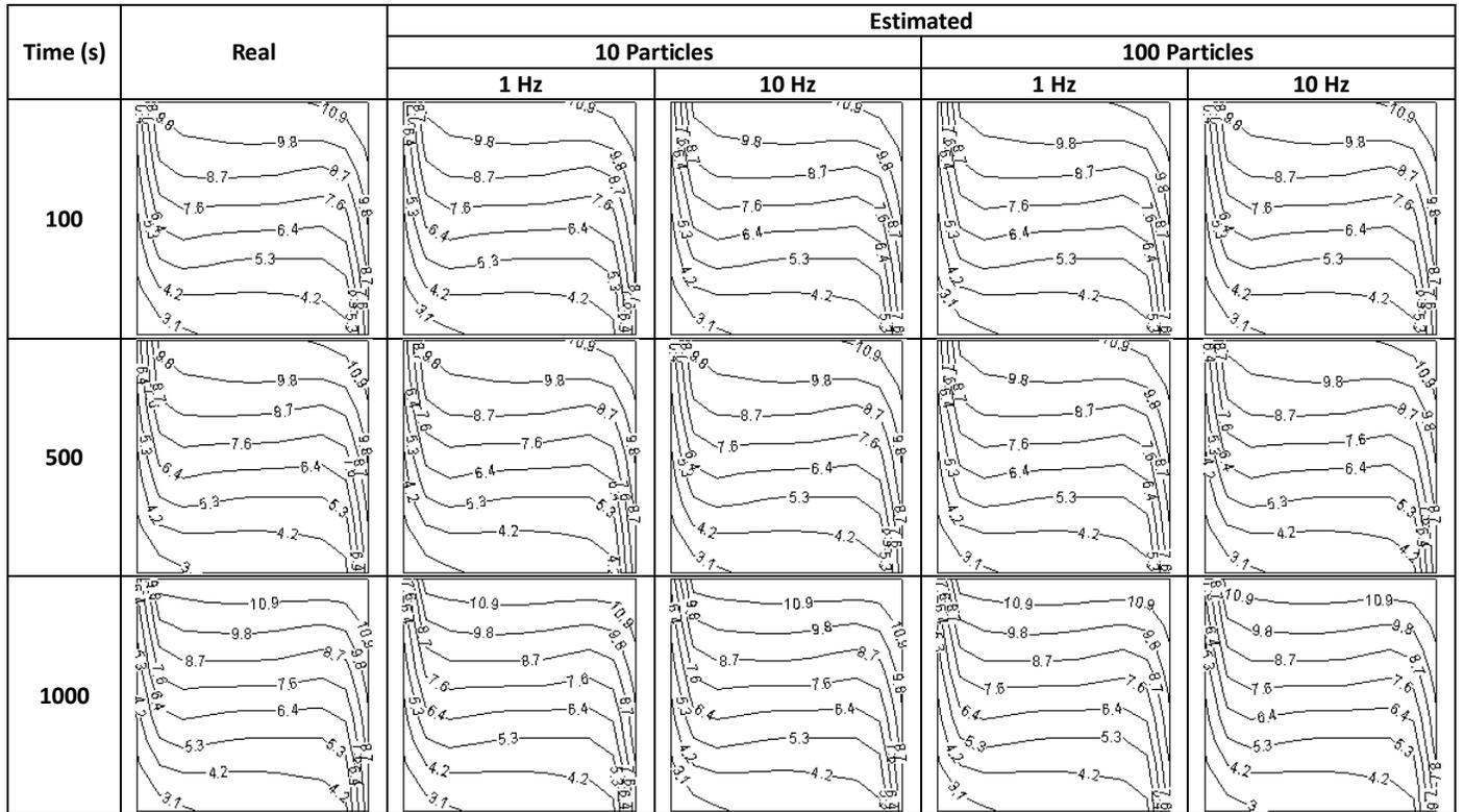
Figure 6 - Real and estimated temperature profiles with the step heat flux profile
