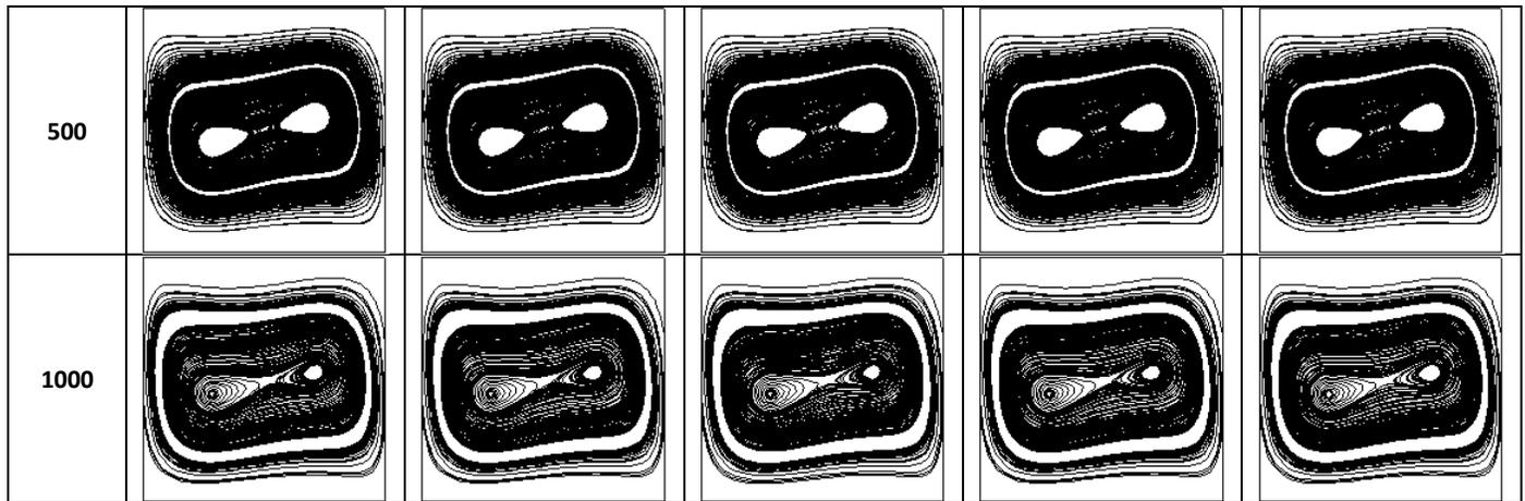
Figure 7 - Real and estimated streamlines with the step heat flux profile
