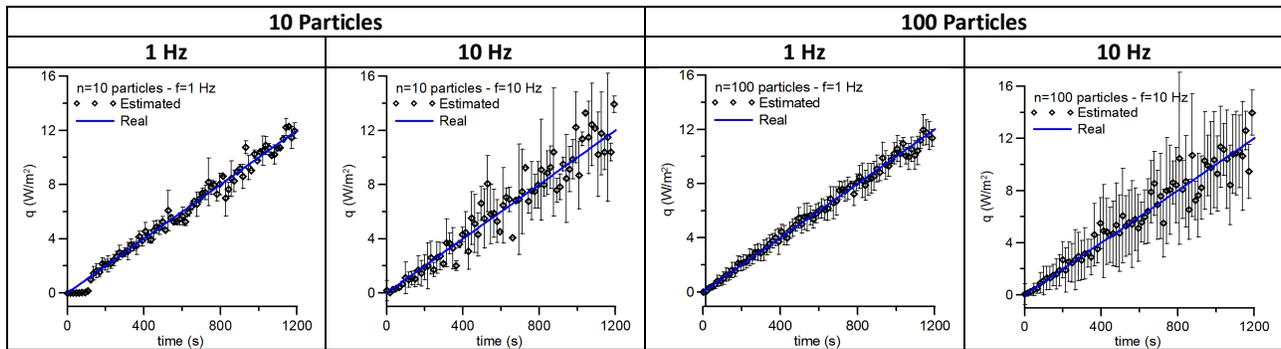
Figure 2 - Estimated heat flux with the linear profile
