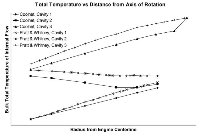
Fig. 6: Comparison of distribution of total temperatures of internal coolant flow predicted by COOLNET vs Pratt & Whitney internal flow analysis code calibrated for F100 second blade
