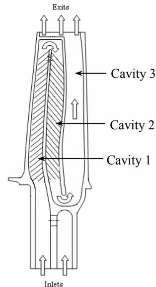
**Fig. 1:** Cross-section schematic of an internally cooled object (a gas turbine blade) depicting cavities, global direction of coolant flow, turbulator ribs, turn-around sections, inlets and exits
