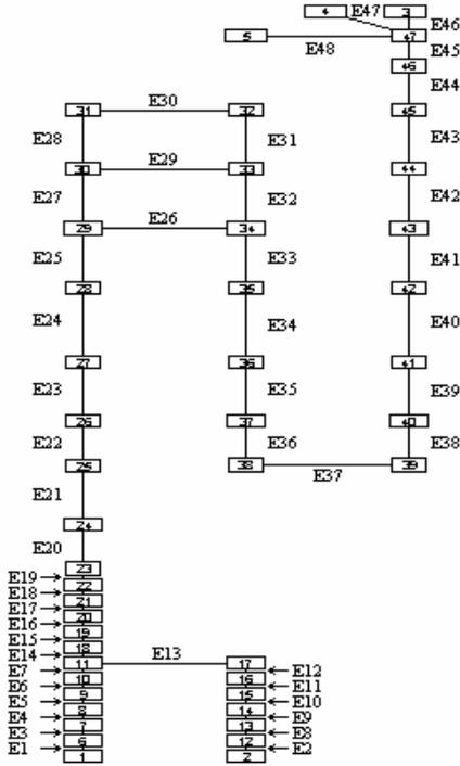
**Fig. 2:** Coolant passage network model for the internally cooled turbine blade
