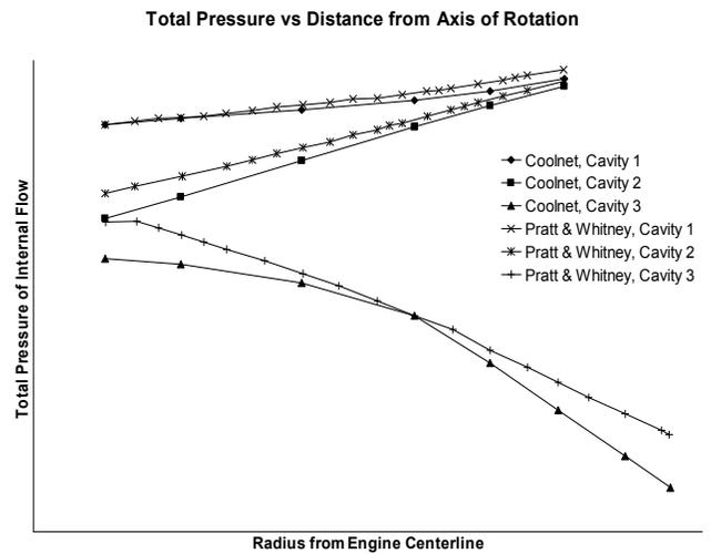
Fig. 5: Comparison of distribution of total pressures of internal coolant flow predicted by COOLNET vs Pratt & Whitney internal flow analysis code for F100 second blade.
